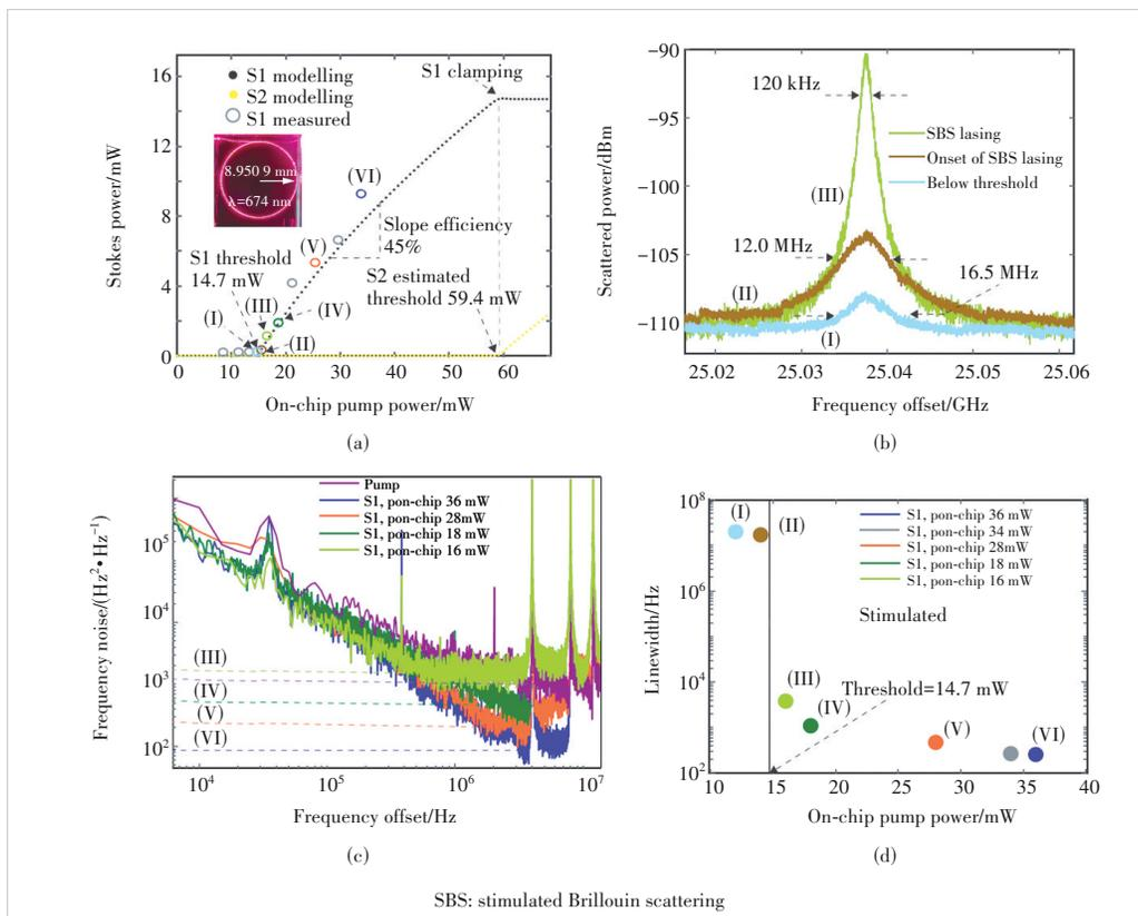
▲ Figure 7. Measurements of the Stokes threshold, power, and linewidth of the 674 nm SBS laser<sup>[95]</sup>
