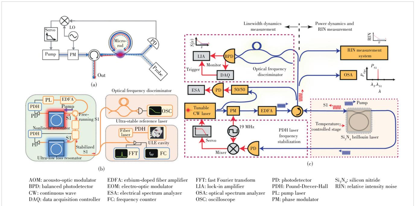
▲ Figure 5. (a) Measurement setup of Brillouin laser loaded Q<sup>[68]</sup>; (b) Brillouin laser stabilization and frequency noise measurement<sup>[90]</sup>; (c) measurement setup of Brillouin laser linewidth, phase noise, relative intensity noise (RIN) and power dynamics<sup>[71]</sup>
