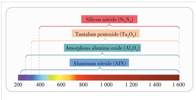
▲ Figure 1. Next generation optical waveguide platforms and wavelength transparency based on the bandgap ( $\text{Si}_3\text{N}_4$ ,  $\text{Ta}_2\text{O}_5$ ,  $\text{Al}_2\text{O}_3$ , and  $\text{AlN}$ )<sup>[49]</sup>
