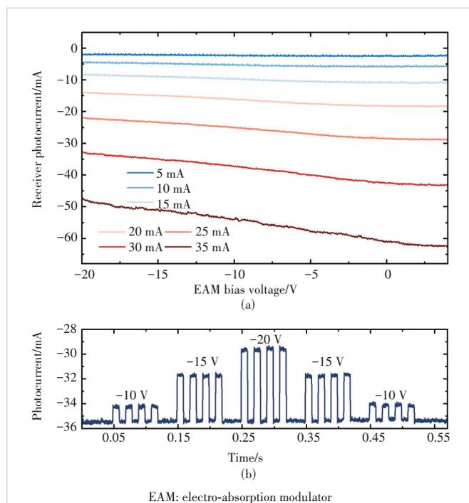
▲ Figure 6. (a) Photocurrent change of the receiver as the voltage biased on the modulator varies with the transmitter under different operating currents; (b) waveforms of the receiver's photocurrent when EAM is modulated
