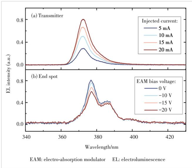
▲ **Figure 4.** (a) Electroluminescence spectra of the LED with several different injection currents; (b) spectra of the end spot when the EAM is under different modulation voltages
