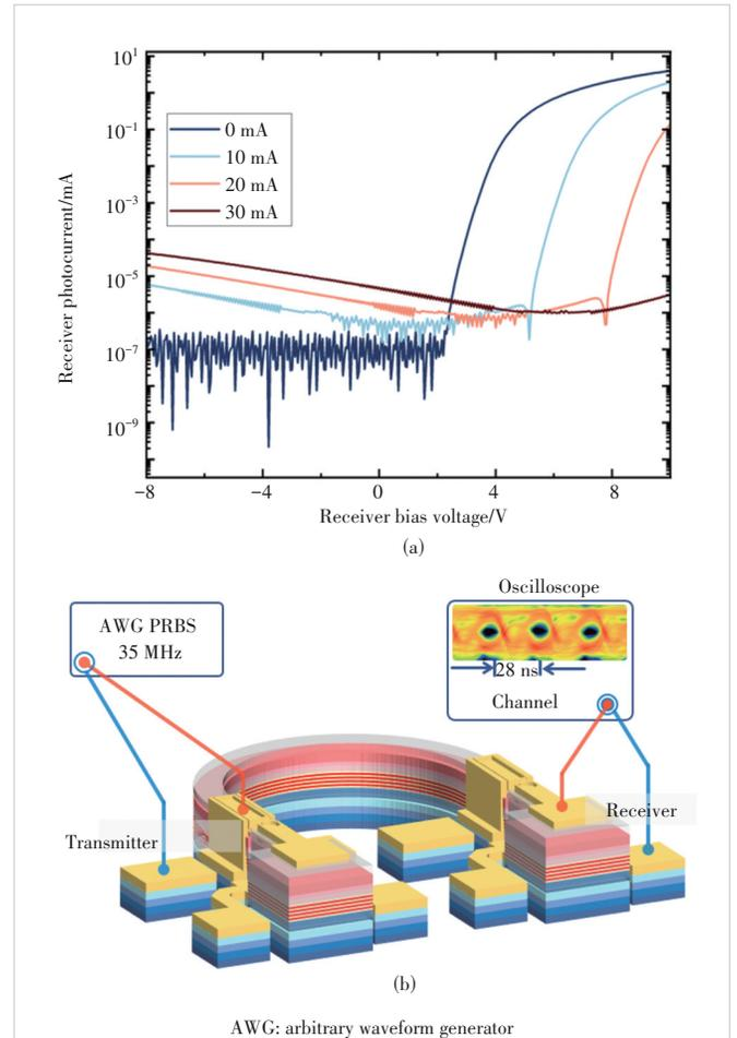
▲ **Figure 5.** (a) Receiver photocurrent versus applied voltage at different transmitter injection currents; (b) 35 Mbit/s on-chip data transmission test with emission modulation mode
