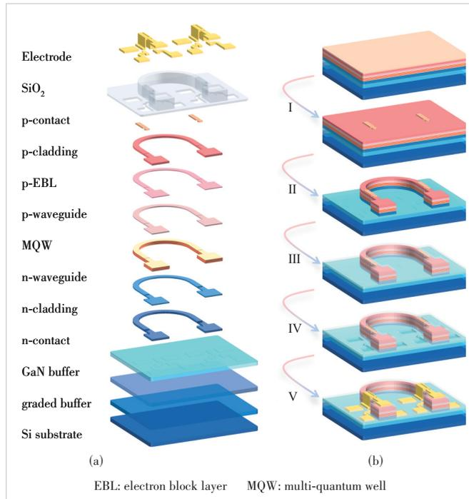
▲ Figure 1. (a) Layered structure of the III-nitride-on-Si optoelectronic system integrated with a 180° bent waveguide; (b) diagram of the top-down manufacturing process
