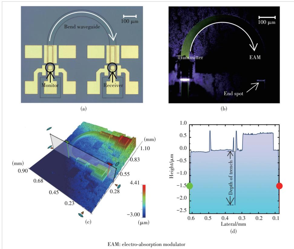
▲ Figure 2. (a) Birdview of the on-chip system under an optical microscope; (b) luminescence image of the optoelectronic chip; (c) characterization of the mesa height using a stylus profilometer; (d) height characterization along the cross-section in (c)
