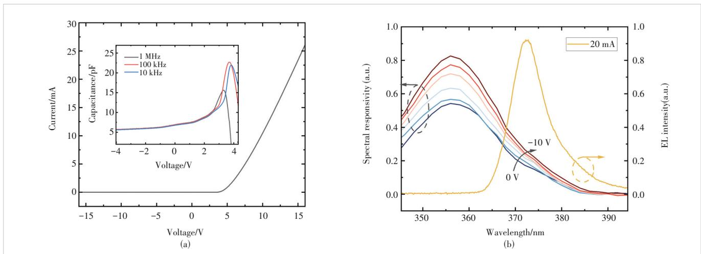
▲ Figure 3. (a) I-V curve of the transmitter, where the inset is the capacitance-voltage curve of the EAM; (b) electroluminescence spectrum and spectral responsivity curves of optoelectronic chip
