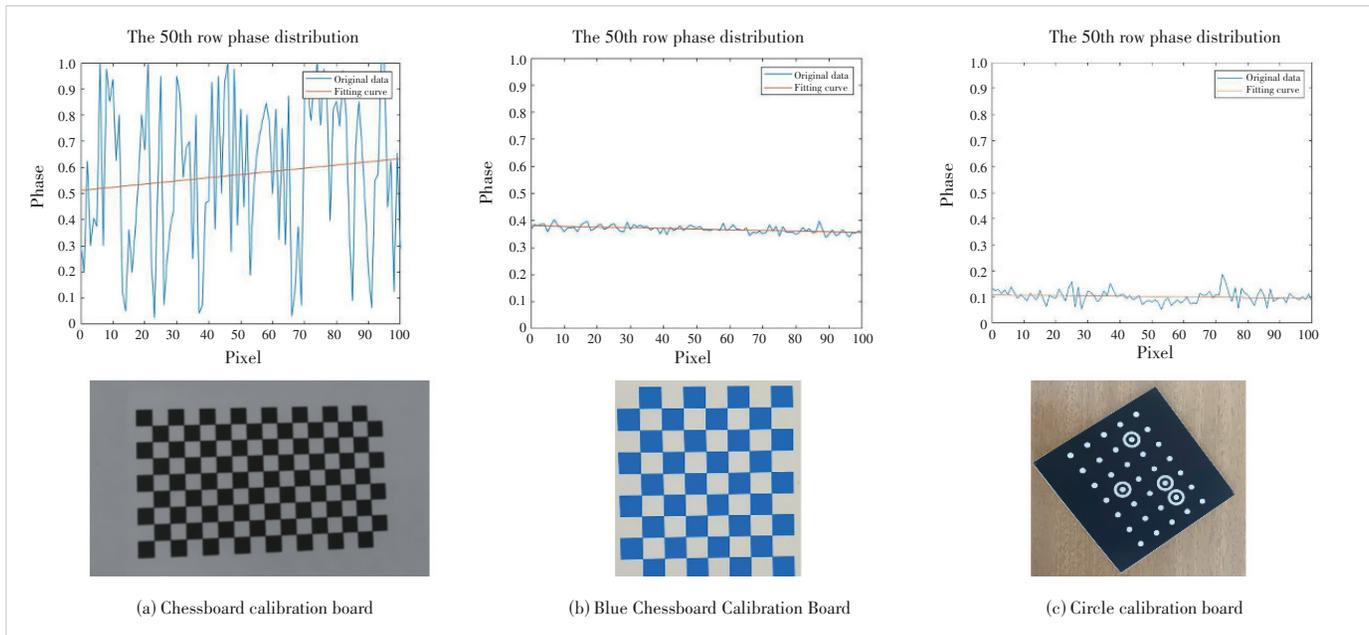
▲ Figure 2. Different calibration board’s phase distribution
