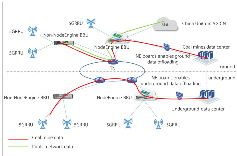
Figure 5-2 Shanneng Group NodeEngine private network solution provides local private network application for the services under the mine
