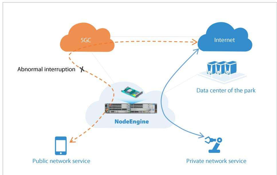
Figure 4-5 Independent operation in isolated scenarios, services not interrupted
